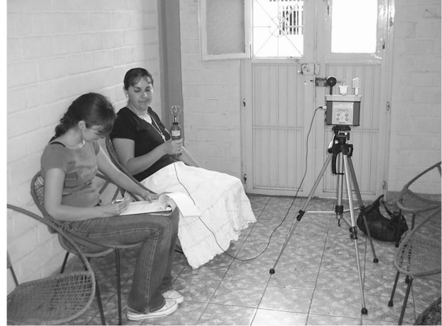
Figure 2. Students apply a questionnaire and adjust the monitor of thermal stress inside a low cost housing unit, at Colima.
